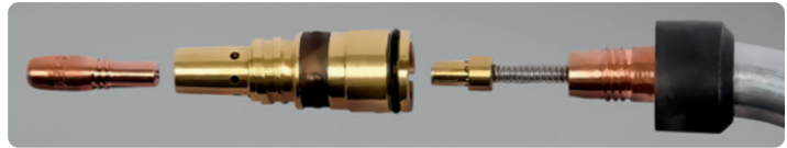
Front-loading AccuLock liner locks at front and back of gun to align with contact tip and power pin for a flawless wire-feed path (AccuLock S consumables shown)
