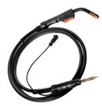
HR-100 Replacement MIG Gun 284546 Comes in 10 ft. (3 m) length with liner for .030-.035 in. (0.8-0.9 mm) diameter wire.
