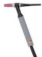
PTA-26, PTA-26V, PTA-26F and PTA-26FV Air-cooled TIG torch, rated 200 amps at 60% duty cycle. The PTA-26V is equipped with a valve for gas flow control. The PTA-26F is equipped with a flexible head for easy maneuverability into tight spaces. The PTA-26FV is equipped with both a gas valve and flexible head.
