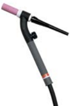
PTA-17, PTA-17V, PTA-17F and PTA-17FV Air-cooled TIG torch, rated 150 amps at 60% duty cycle. The PTA-17V is equipped with a valve for gas flow control. The PTA-17F is equipped with a flexible head for easy maneuverability into tight spaces. The PTA-17FV is equipped with both a gas valve and a flexible head.
